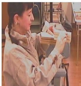
This shot shows the progression as Carlyn hollows out the box carefully measuring the depth. She made quite a lot of use of a negative rake scraper in the hollowing process. After finishing the inside and top of the outside, she reversed it on the chuck using a jam chuck. This enabled her to finish the bottom. Leaving a small spigot on it to take a foot.
