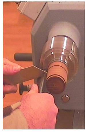
Steve then proceeded to part the lid from the body using a thin parting tool. Steve prefers to hollow out the lid first fitting the body spigot to the lid. After facing it off, taking note of the depth he had available, he hollowed out the lid with a spindle gauge, finishing it off with a negative rake scraper. Aligning the tool with the bed bars to get parallel walls.
