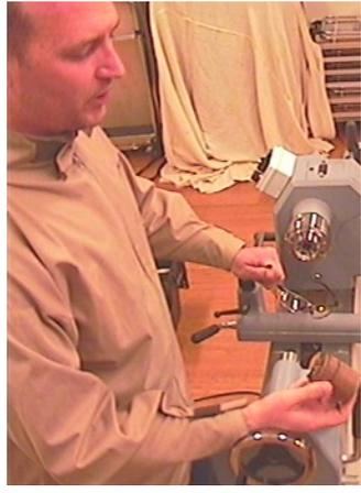
Steve then set about hollowing out the body of the box. Taking care to get the right depth he made sure the sides were straight by once again aligning the tool with the bed bars. When he was satisfied with the depth and finish he removed it from the chuck, and replaced it with a piece of scrap wood to make a jam chuck so he could reverse the box body and finish the bottom.
