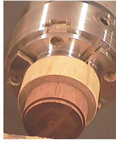
This picture shows the jam chuck Steve made to hold the body securely whilst finishing of the bottom of the box. As you can see, Steve made a first class job of the fit, and proceeded to finish the bottom of the box. And put a shallow concave finish to it so that it sat properly on a table..
